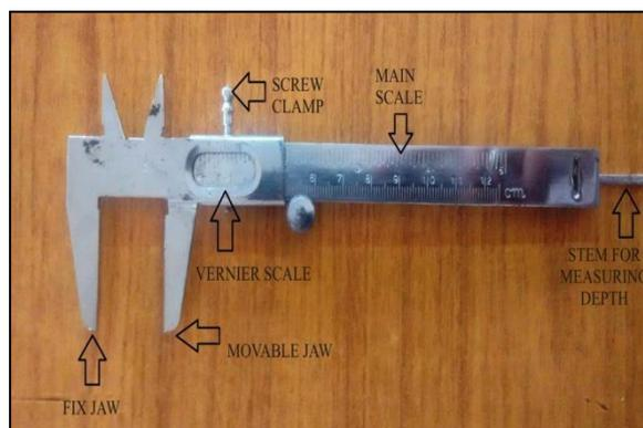
Fig-1: Sliding Verneir caliper
