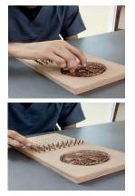
Figure 3: O'Connor Finger Dexterity Test (OCFDT)
